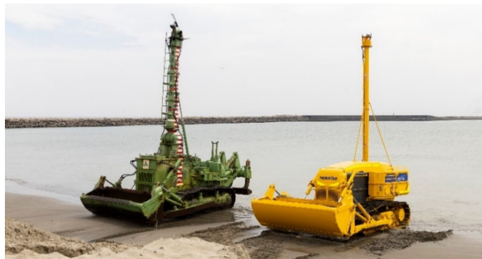
[Amphibious bulldozer (left) and underwater construction robot under field trials (right)]
